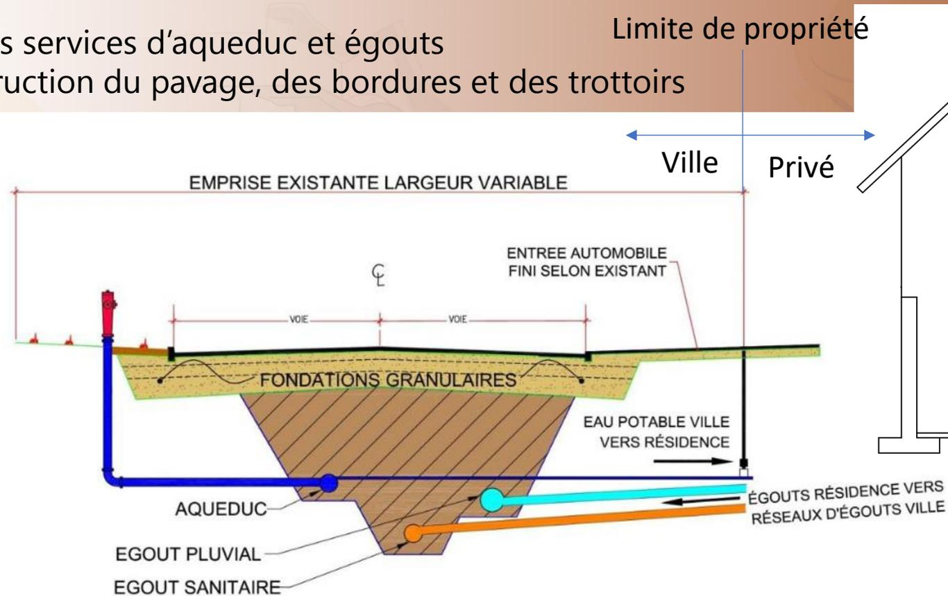
FIGURE: RECONSTRUCTION DE LA CHAUSSÉE AVEC AQUEDUC, ÉGOUT DOMESTIQUE ET ÉGOUT PLUVIAL.
